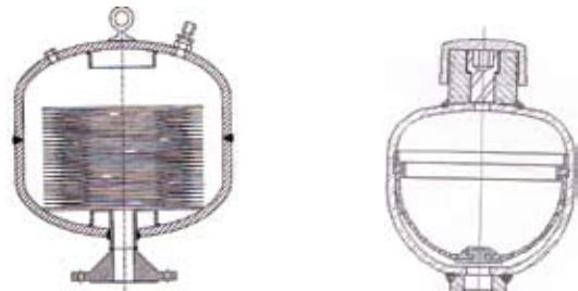
**Because metal bellow type dampeners are relatively expensive, they are used for very high temperatures or extreme compatibility applications, such as those in the pharmaceutical industry.**
